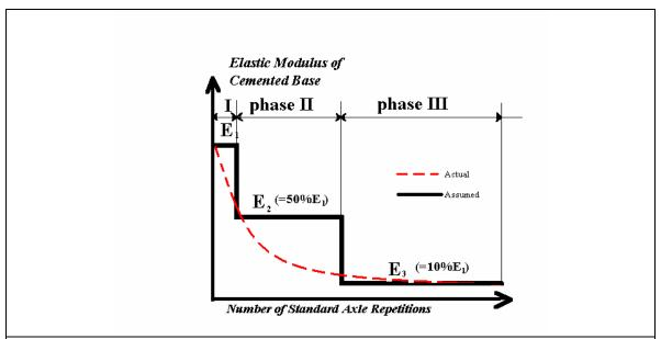
Figure-2: Varaiation of elastic modulus of the cemented layer with traffic repetitions (Das and Pandey 1998)
