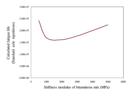
**Figure 1** Variation of calculated fatigue life with stiffness modulus of bituminous mix.
