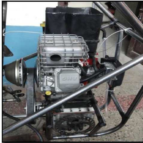
Figure 4.36: Briggs and Stratton engine coupled with a CVT. Image source: Vehicle design report [71].
