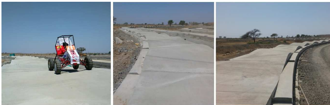
Figure 4.35: Low severity (left), medium severity (middle) and high severity (right) chassis twist test tracks respectively.
