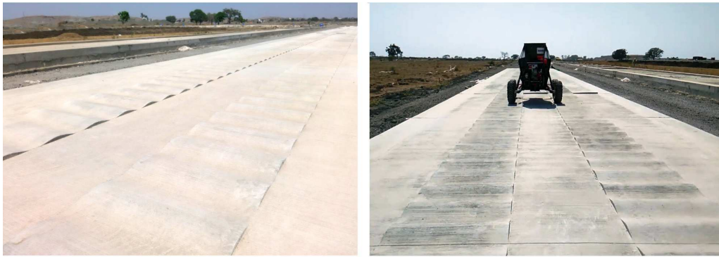
Figure 4.63: Left: sinesweep track (the decreasing wavelength is visible); Right: vehicle on the sinesweep track.
