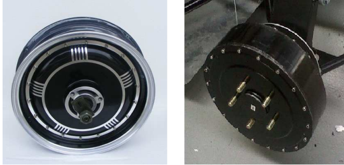
Figure 2.19: The vehicle is equipped with Kelly 72V - 7KW wheel hub motors (left) weighing 46 kg each which leads to an overall front and rear unsprung mass of 60 kg and 65 kg respectively (see Table 2.3). The hub motor assembly on one of the wheels is shown on the right. Image source: Kelly controls LLC [40].
