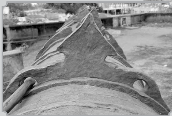
Figure C. Details of one of the handling clamps.
