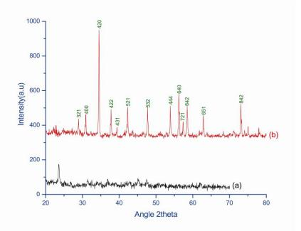
Powder XRD of laser sintered Ce:YAG.
