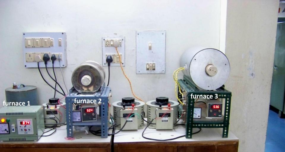
Temperature ± 1 °C furnace 1: 500 °C max; air furnace 2: 1200 °C max; air Furnace 3: 1200 ° C max; oxygen/nitrogen/He
