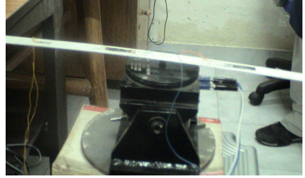
Figure 11. Experimental set-up is showing two IPMC patches on the link and the exciter.
