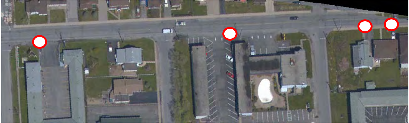
Figure 77: Power line points are detected and displayed over ortho photo in view 2
