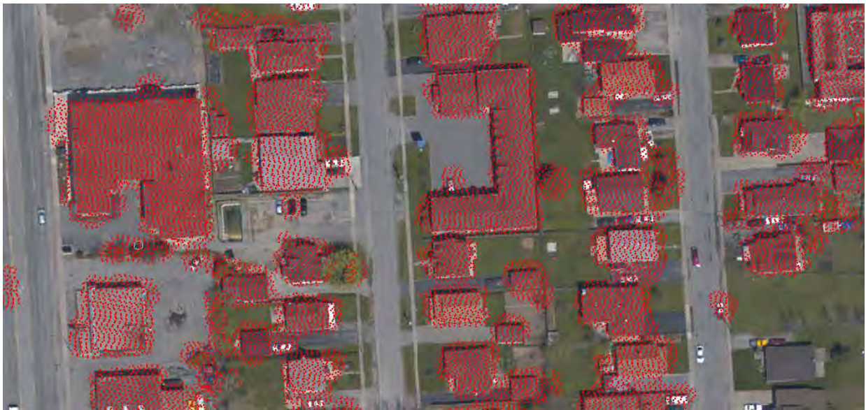
Figure 32: Classified building points displayed over ortho photo
