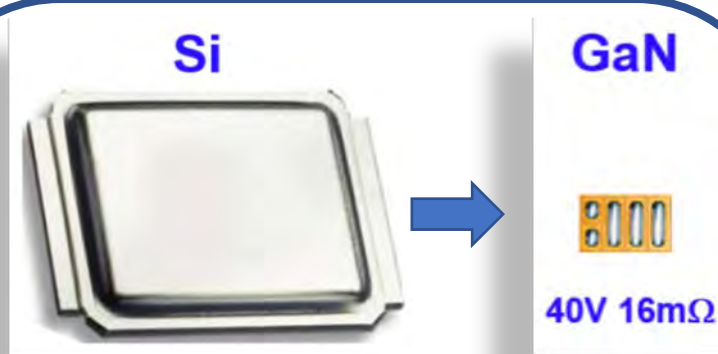
Size comparison of Si power MOSFET with GaN HEMT from EPC for same performance
