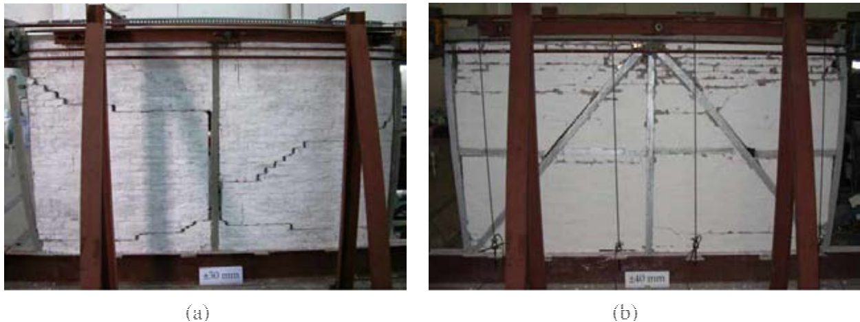
Figure 4 (a) Specimen 1 and (b) Specimen 2 at the conclusion of the test
