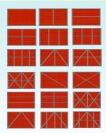
Confinement Fator (i/t) is ratio of total length of internal grid elements (i) divided by total length of boundary confining elements (t).
