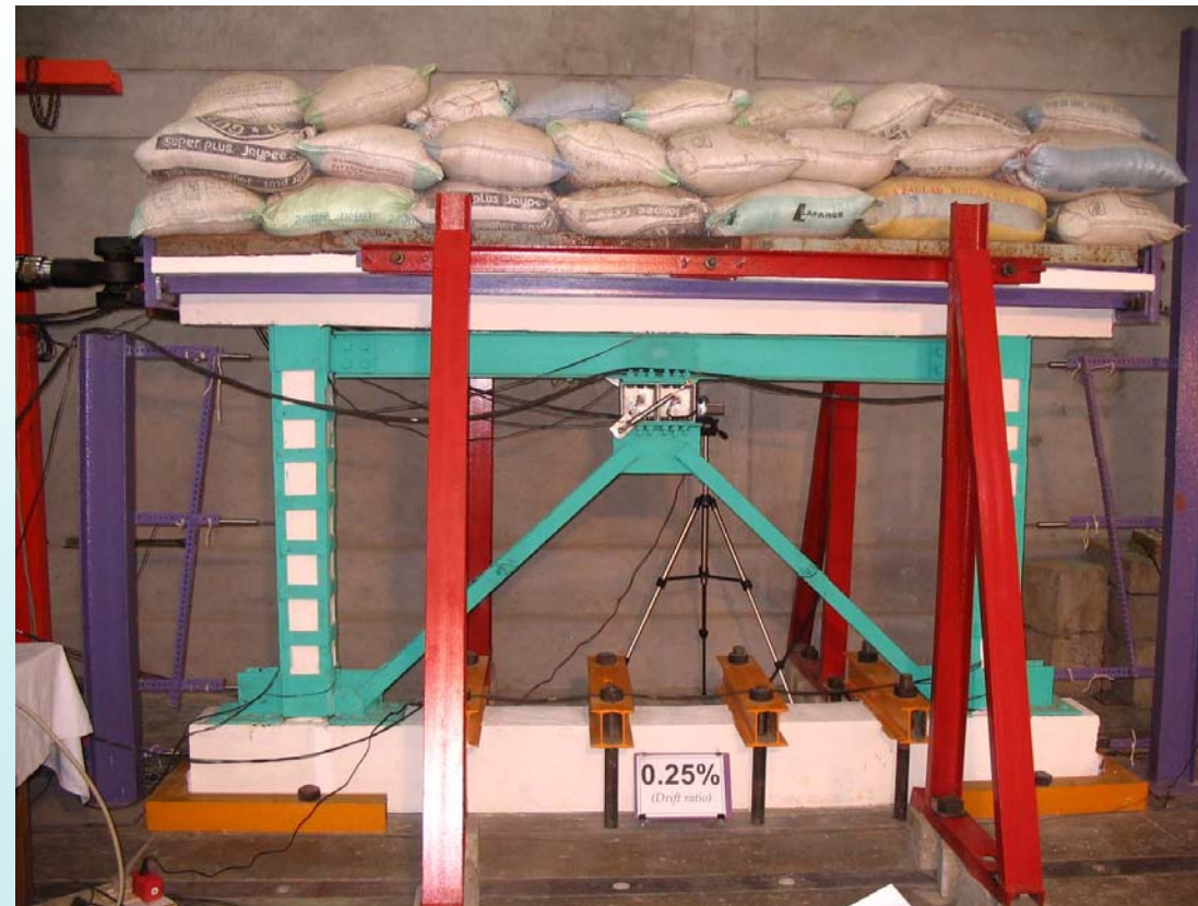
Single-story single-bay reduced scale (1:0.4) RC frame subjected to gravity loads and reversed cyclic lateral displacements as per ACI-374 seismic testing loading protocol
