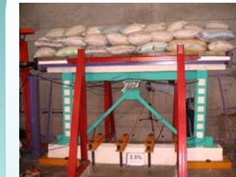
State of strengthened frame at 3.5% drift
