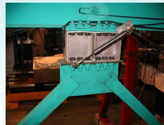
Arrangement of AI-SYD in strengthened frame
