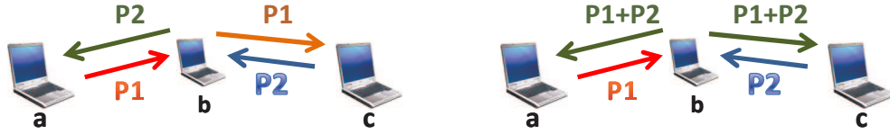
Figure 1.1: Information exchange through a relay node. Colors index the different time slots.
