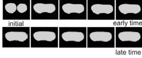
Fig. 4: Footprint of coalescence of pendant drops of equal volume ( v_1 = 0.03 \mu\text{l} v_2 = 0.03 \mu\text{l} ) on a Teflon substrate with an equilibrium contact angle of 90^\circ
