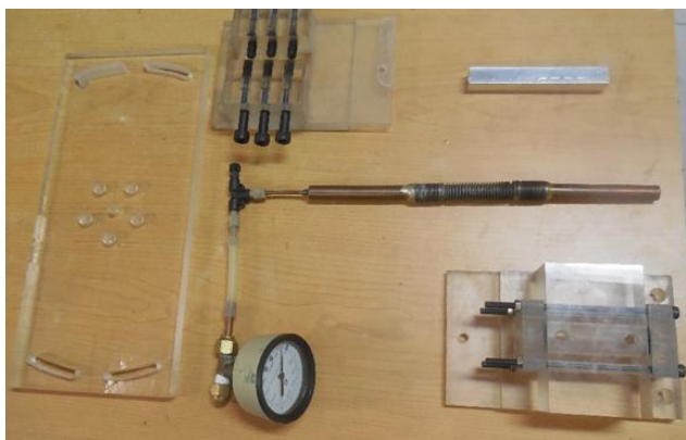
FIGURE 1: The developed flexible heat pipe and the components manufactured for its testing.
