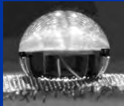
8µl drop on untreated SS#200 mesh CA ~ 120°
