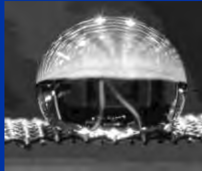
8µl drop on untreated SS#100 mesh CA ~ 120°
