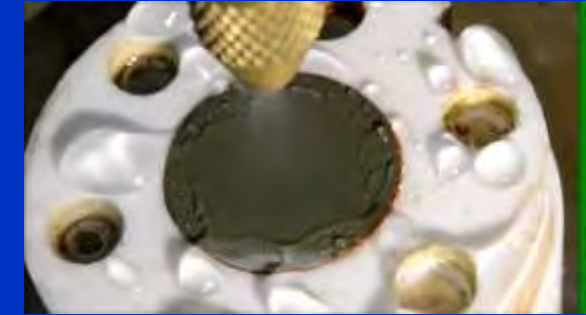
Effect of surface morphology on spray impingement
