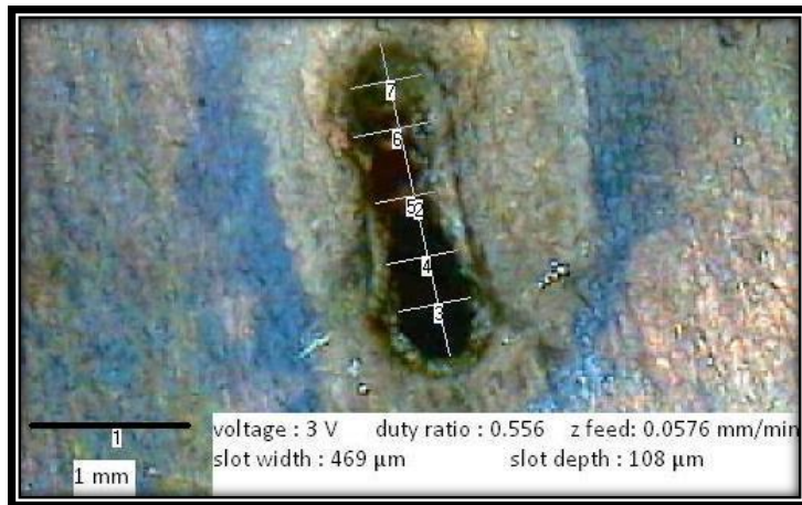
Slots machined with uncoated tool
