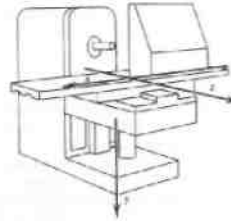
Figure 10.4 Coordinate system for a mill. (Y. Koren, Computer Control of Manufacturing Systems , McGraw-Hill, 1983.)
