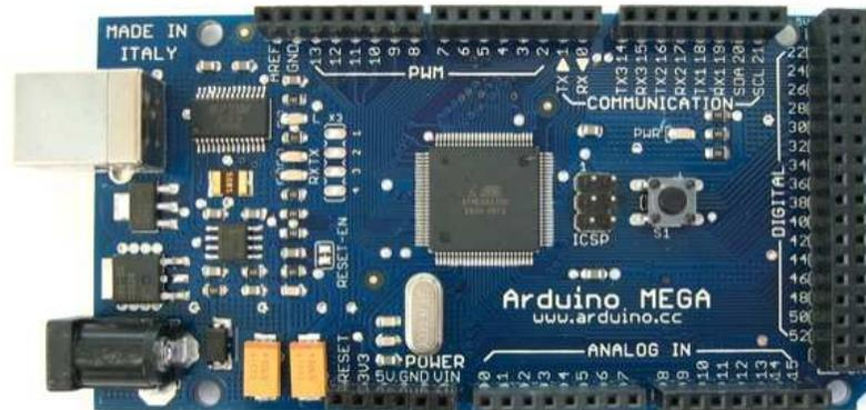
**POWER:** The Arduino Mega can be powered via the USB connection or with an external power supply. The power source is selected automatically.
