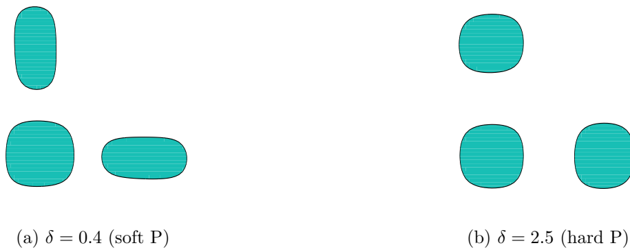
Figure 7: Equilibrium shape of three, initially circular and same-sized, precipitates ( l = 30 nm) with anisotropic interfacial energy density and isotropic bulk elasticity.
