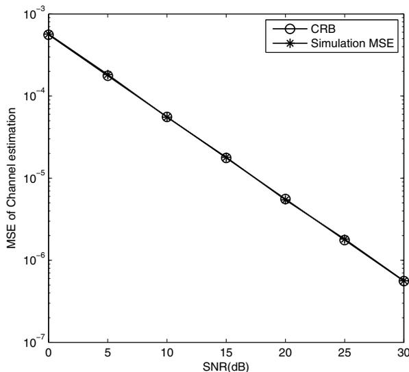
Fig. 4. The MSE performance of the channel estimator
