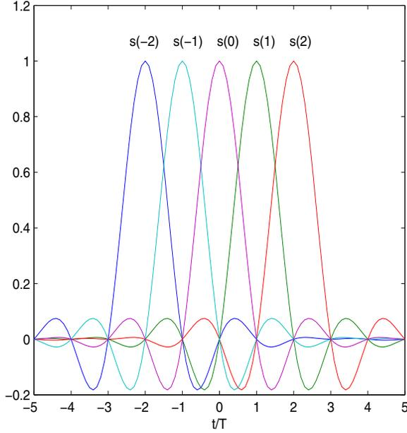
Fig. 2. Individual contributions of  $s(n)$  on the transmitted signal  $c(t)$
