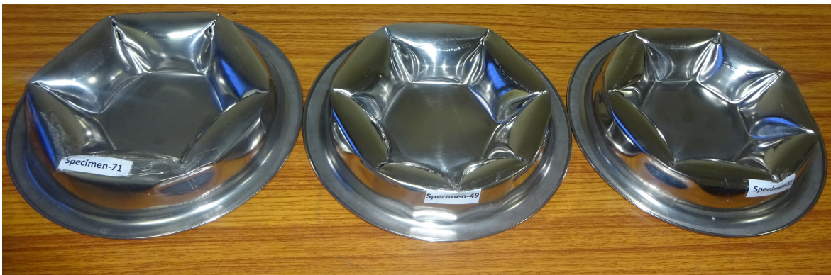
Figure 2.15: Bowl deformed shapes. Left: Minimum buckling load (1.91 kN). Center: Median buckling load (3.39 kN). Right: Maximum buckling load (4.91 kN). The wave numbers observed are 6, 7, and 7.
