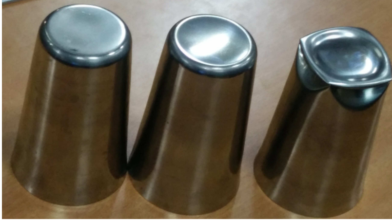
Figure 2.11: Left: three stages of tumbler deformation. The depression caused in the flat base is due to plastic deformation near the periphery. The light source was arranged to aid visibility by reflection.
