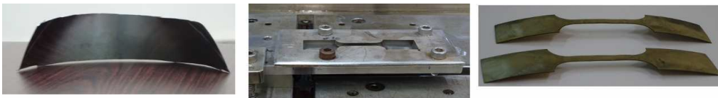
Figure 2.7: Cutting procedure for tensile specimens from bowls.
