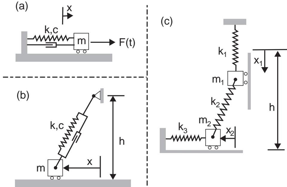
Figure 2: (a) A linear, damped, forced system. (b) A nonlinear system. The spring has a free length  $L_0 > h$ . (c) A nonlinear two degree of freedom system. Mass  $m_1$  is constrained to move frictionlessly in the vertical direction, while mass  $m_2$  moves in the horizontal direction. Gravity is neglected, for simplicity.
