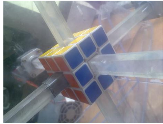
Shaft alignment and attachment
