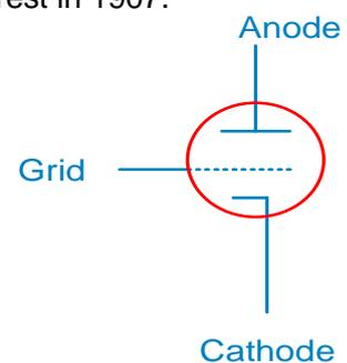
Schematic diagram of a Triode
