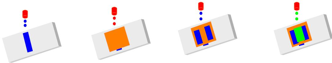
Schematic illustrating fabrication of a transistor using Printing
