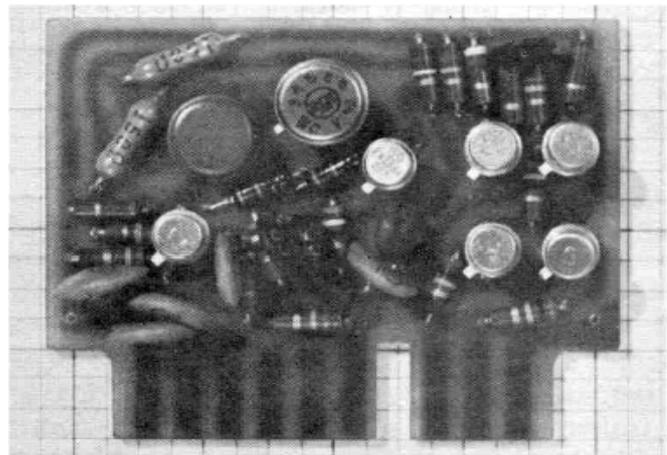
**P45, an early operational amplifier built using discrete transistors**
