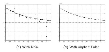
Figure: Solutions of a mass-spring-damper system: stiff situation
