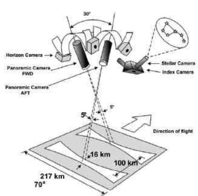
Figure 1. Imaging geometry of CORONA KH-4B camera<sup>20</sup>.
