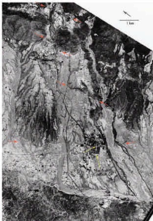
**Figure 4.** CORONA satellite photograph of the area around Pinjore town located about 25 km NE of Chandigarh in NW Himalaya. Active fault traces are marked by red arrows<sup>23</sup>.
