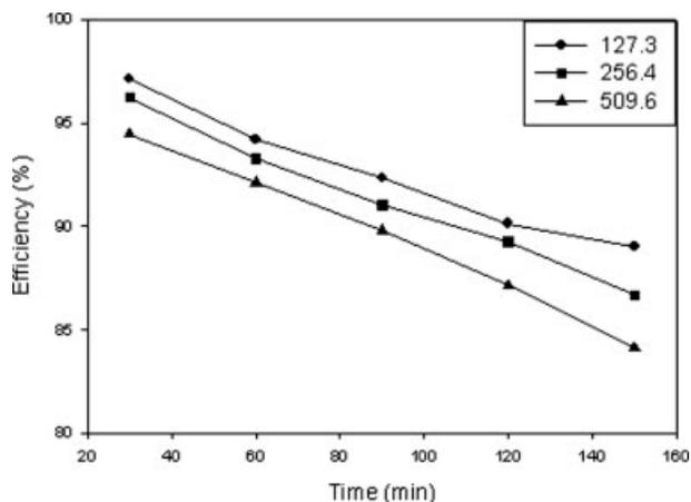
**Figure 8.** Variation of current efficiency for AEM with time at different current densities,  $\text{A/m}^2$  (salt concentration = 4.2 N, flow rate = 66 ml/min, HCl concentration 0.5 N, temperature =  $25^\circ\text{C}$ ).
