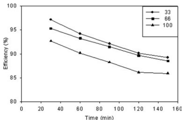
**Figure 10.** Variation of current efficiency for AEM with time at different circulation rates, ml/min (current density =  $254 \text{ A/m}^2$ , salt concentration = 4.2 N, HCl concentration 0.5 N, temperature =  $25^\circ\text{C}$ ).
