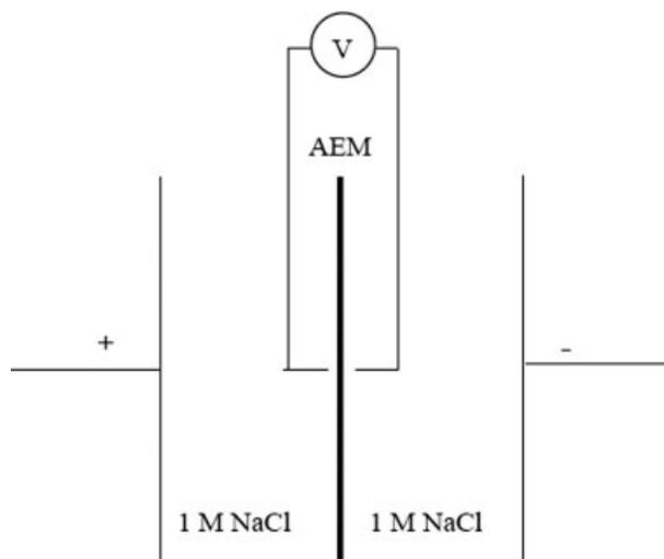
**Figure 2.** Cell arrangement for measuring the potential drop across the membrane.
