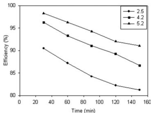
**Figure 9.** Variation of current efficiency for AEM with time at different salt concentrations, N (current density =  $254 \text{ A/m}^2$ , flow rate = 66 ml/min, HCl concentration 0.5 N, temperature =  $25^\circ\text{C}$ ).
