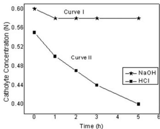
**Figure 7.** Curve I is for the case where both catholyte and anolyte have been filled with 0.6 N NaOH concentration, and indicates that the concentration of  $\text{OH}^-$  ion remains nearly constant in the catholyte.
