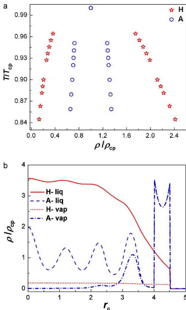
**Fig. 3.** Corresponding state plots of vapor–liquid coexistence envelopes in hard (H) and attractive (A) cylindrical pore of width  $D = 10$  molecular diameters are shown in (a). Typical radial density ( $R$ -density) profiles of coexisting vapor and liquid phases are shown in (b) at a reduced temperature,  $T/T_{cp} = 0.86$ .
