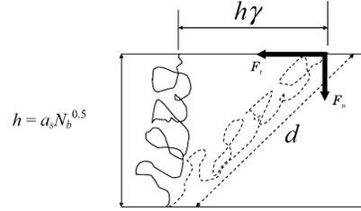
**Figure 2.** Schematic of the polymer chain bridging two opposite layers. The stretching of the same under LAOS can also be seen.
