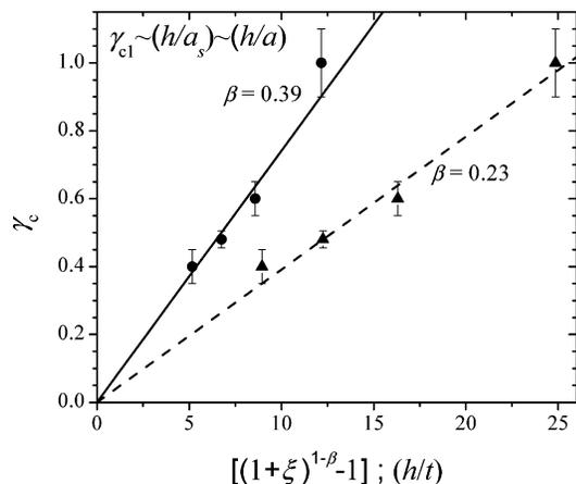
**Figure 3.** Critical strain at the onset of strain hardening plotted against  $(h/t)$ . The points in both data sets are same experimental data for the two values of  $\beta$ , whereas the lines are a linear fit. We get the best linear fits that also pass through an origin for  $0.39 > \beta > 0.23$ .
