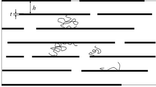
**Figure 1.** Slice of a system in a plane normal to the plane of clay plates. We have assumed that in one layer of thickness of  $t$  the fraction of area occupied by clay plates is given by  $\zeta$ .
