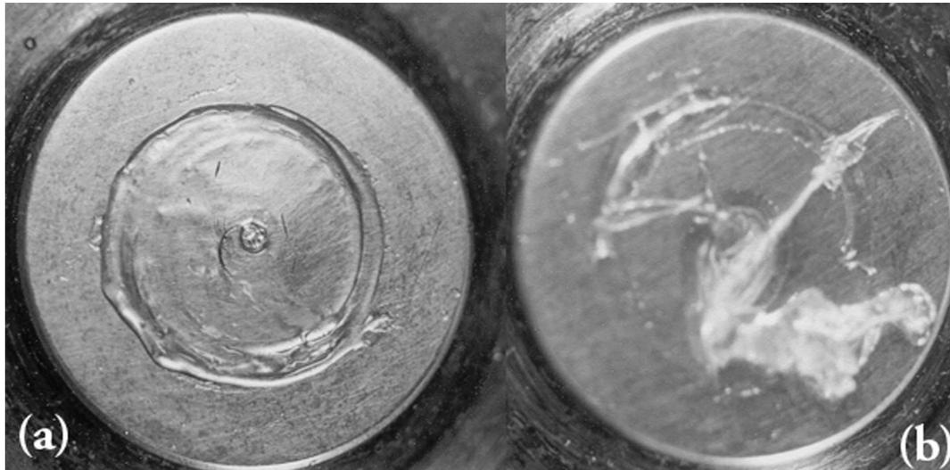
Fig. 2. The photograph of the plate immediately after the instability has occurred in the cone and plate rheometer. The left picture (a) is from the plate where the coated cone was used, while the right picture (b) corresponds to a bare cone. The sample with the coated cone is almost free from distortions relative to the bare cone case.
