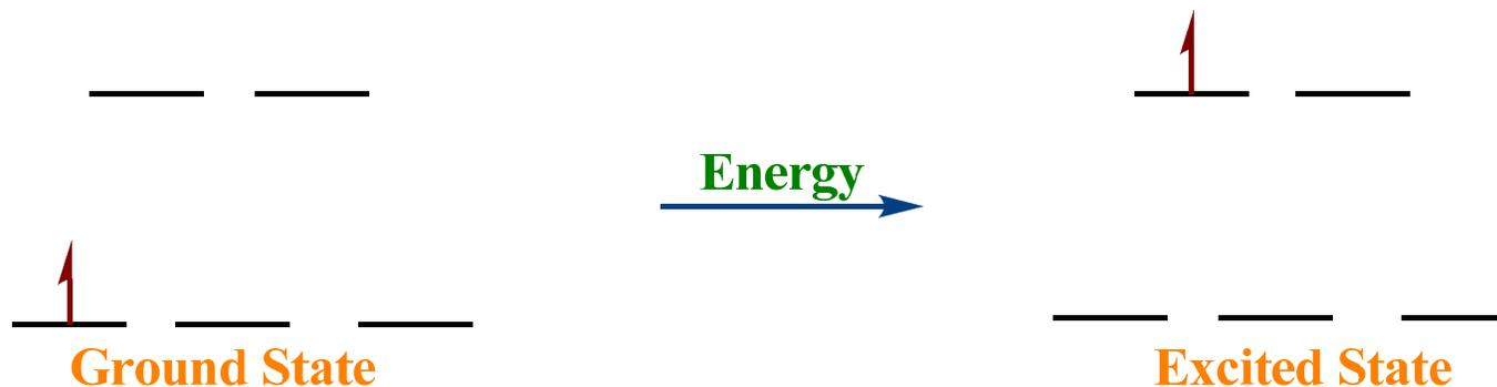
The single electron in the  $t_{2g}$  orbitals absorb energy in the form of light and gets excited to the  $e_g$  orbitals. In case of  $[\text{Ti}(\text{H}_2\text{O})_6]^{3+}$ , this corresponds to 520 nm ( $20,300 \text{ cm}^{-1}$ ).
