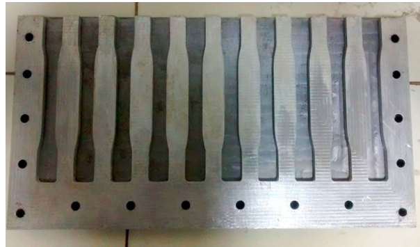
Fig. 3 Mould for making epoxy tensile testing specimen
