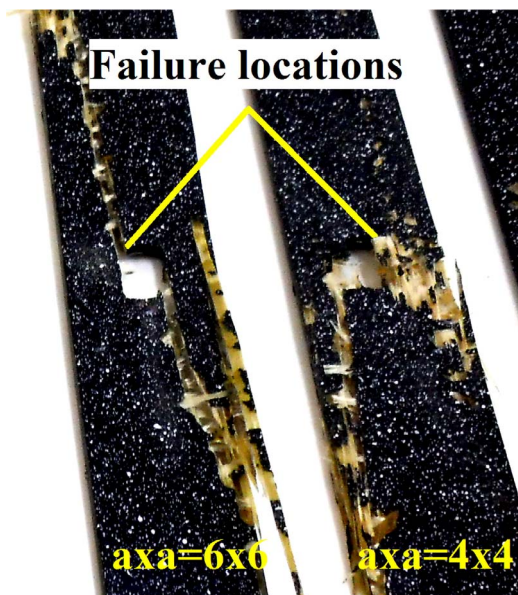
Fig. 25. Final failure of a [0]_4 laminate notched specimens ( a \times a = 4 \times 4 and a \times a = 6 \times 6 \text{ mm}^2 ).
