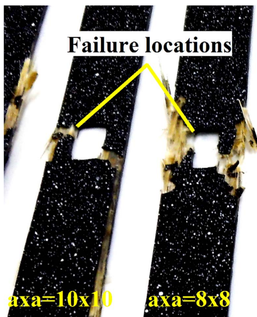
Fig. 28. Final failure of a [0]_4 laminate notched specimens ( a \times a = 8 \times 8 and a \times a = 10 \times 10 \text{ mm}^2 ).
