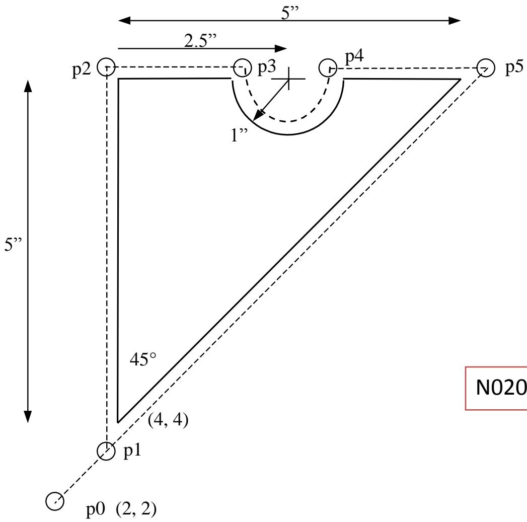
Machine moves in XY-plane
