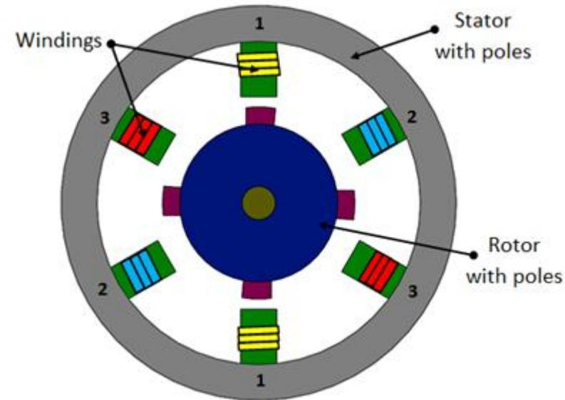
Fig. Variable reluctance stepper motor
