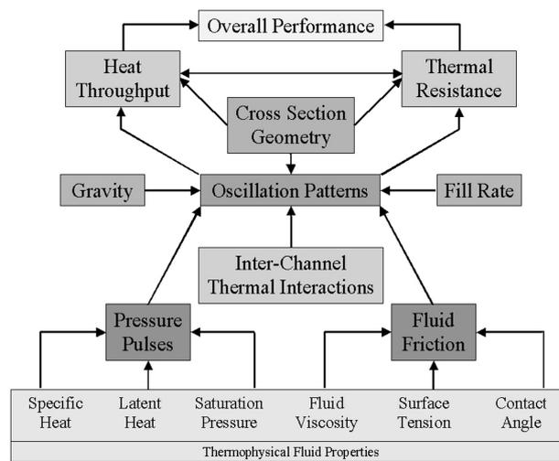
Fig. 3. Parameter dependency chart of a PHP [9]
