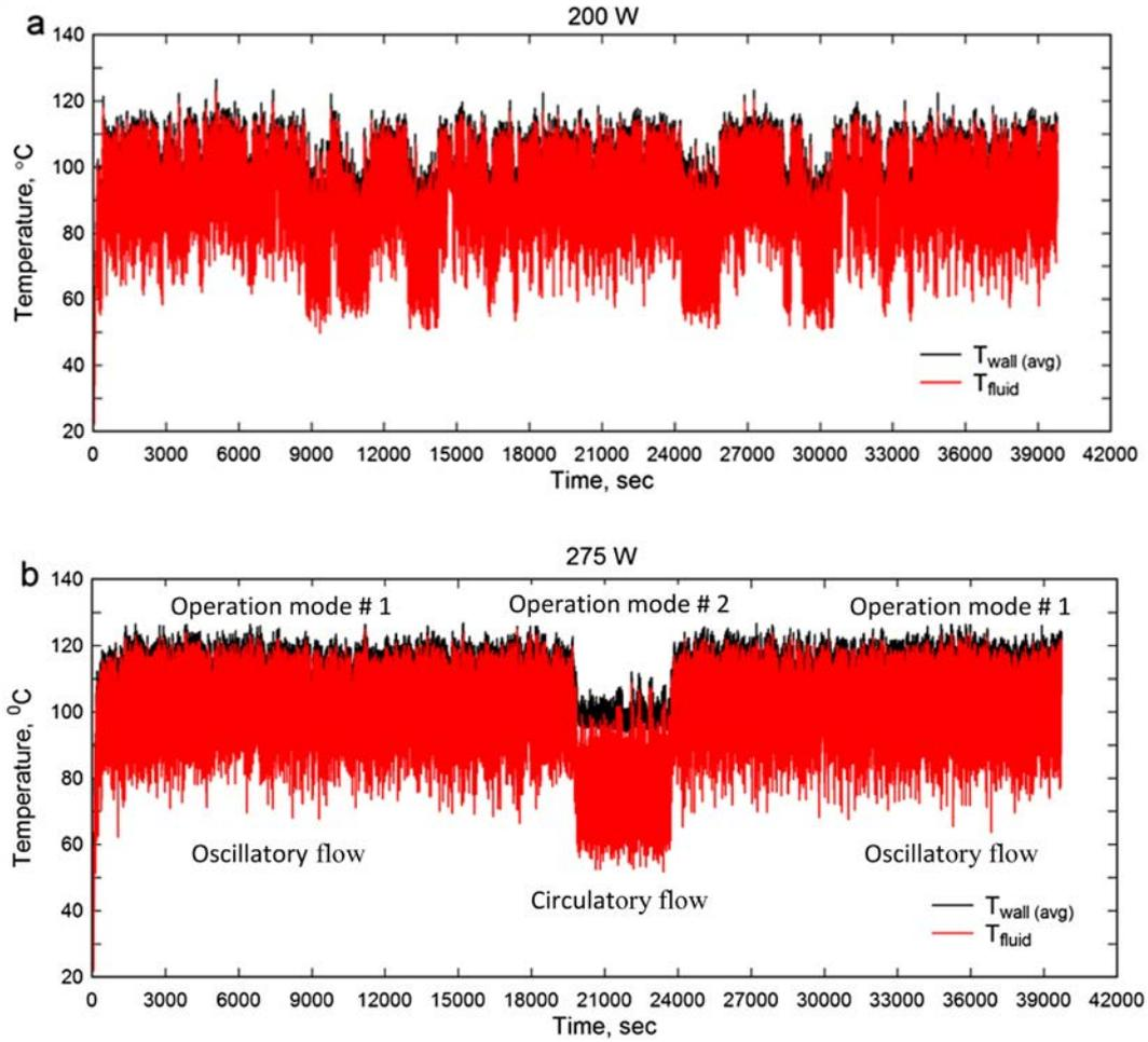
Fig. 6. Multiple pseudo-steady states obtained for different input heat power when the PHP runs continuously for over 11 h (a) at 200 W of heat input and (b) at 275 W of input heat power.
