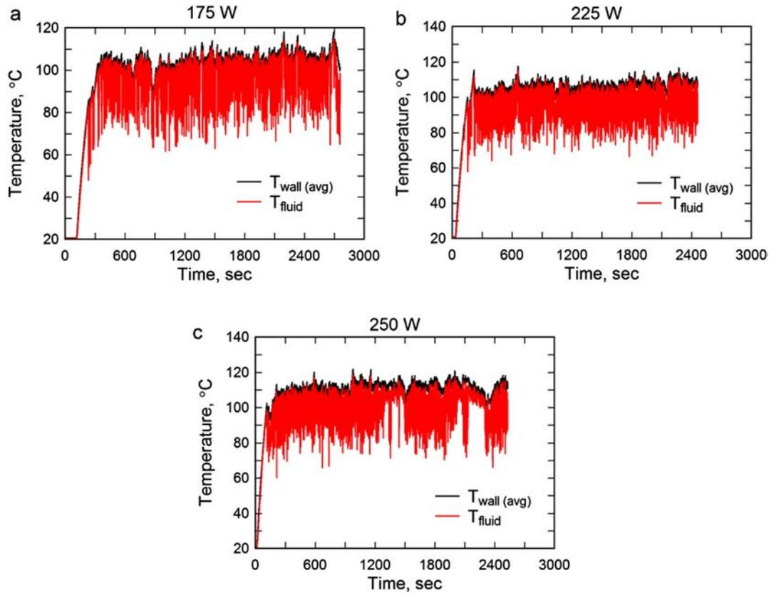
Fig. 3. Temporal evolution of temperature oscillation profiles of wall average and fluid temperatures in the evaporator section for different input heat powers for continuous oscillations of the working fluid.
