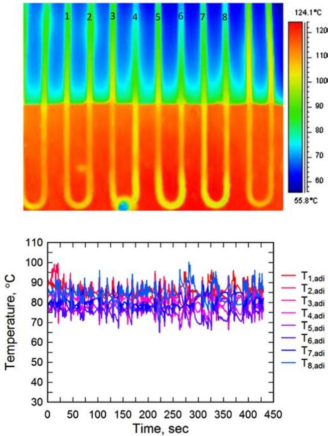
Fig. 8. IR and temperature pulsation profiles during oscillatory flow (Steady-state operation mode #1) at 275 W of input heat power.
