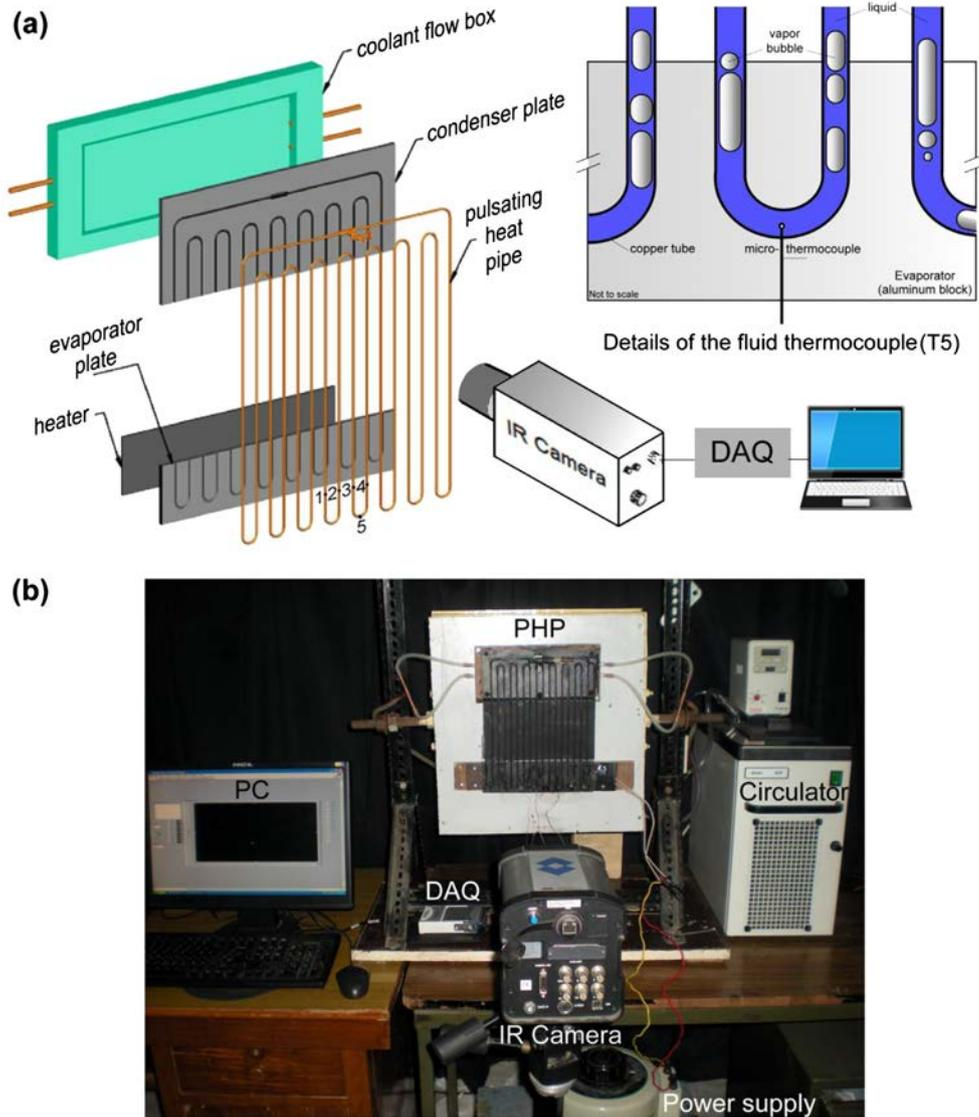
**Fig. 1.** (a) Schematic diagram of the PHP experimental setup along with the details of the thermocouple T5 embedded in the evaporator U-turn for fluid temperature measurement and (b) Photograph of the entire setup with all the peripheral systems.
