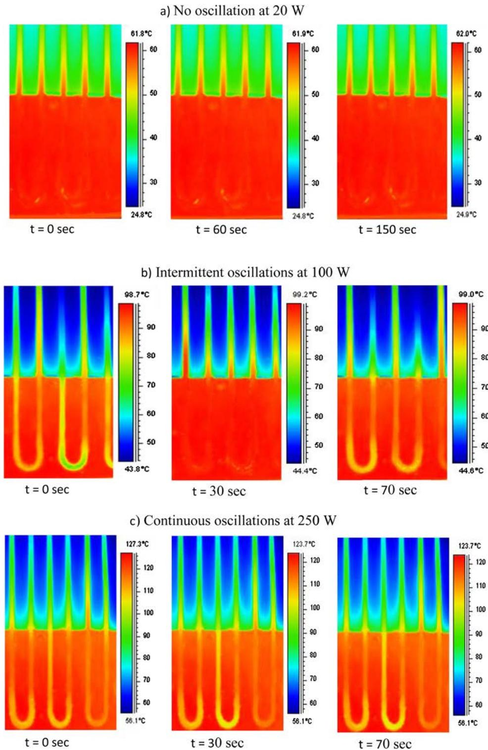
Fig. 4. IR temperature profiles for increasing thermal input power: the temperature scale is given alongside.
