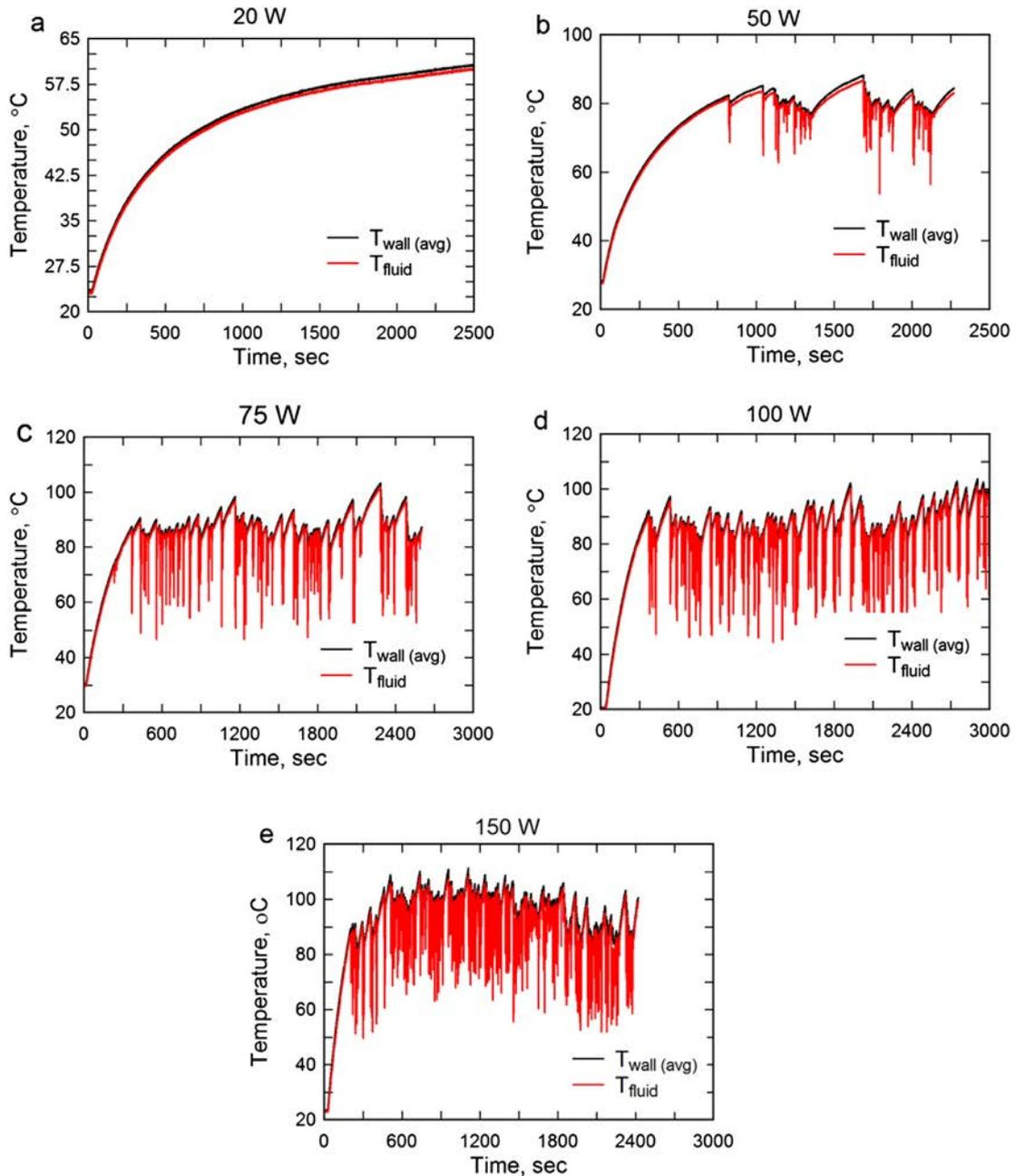
**Fig. 2.** Temporal evolution of temperature oscillation profiles of wall average and fluid temperatures in the evaporator section for different input heat powers (a) no oscillation (b) start-up oscillations and (c) to (e) intermittent oscillations.
