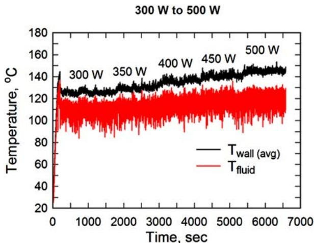
Fig. 9. Time temperature plot of the average evaporator temperature when the PHP was operated at high power (from 300 W till 500 W).
