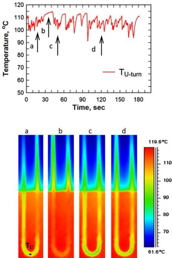
Fig. 5. Temperature oscillation profile and IR thermo-grams of a U-turn in the evaporator at a specified pseudo-steady state for 250 W of heat power.
