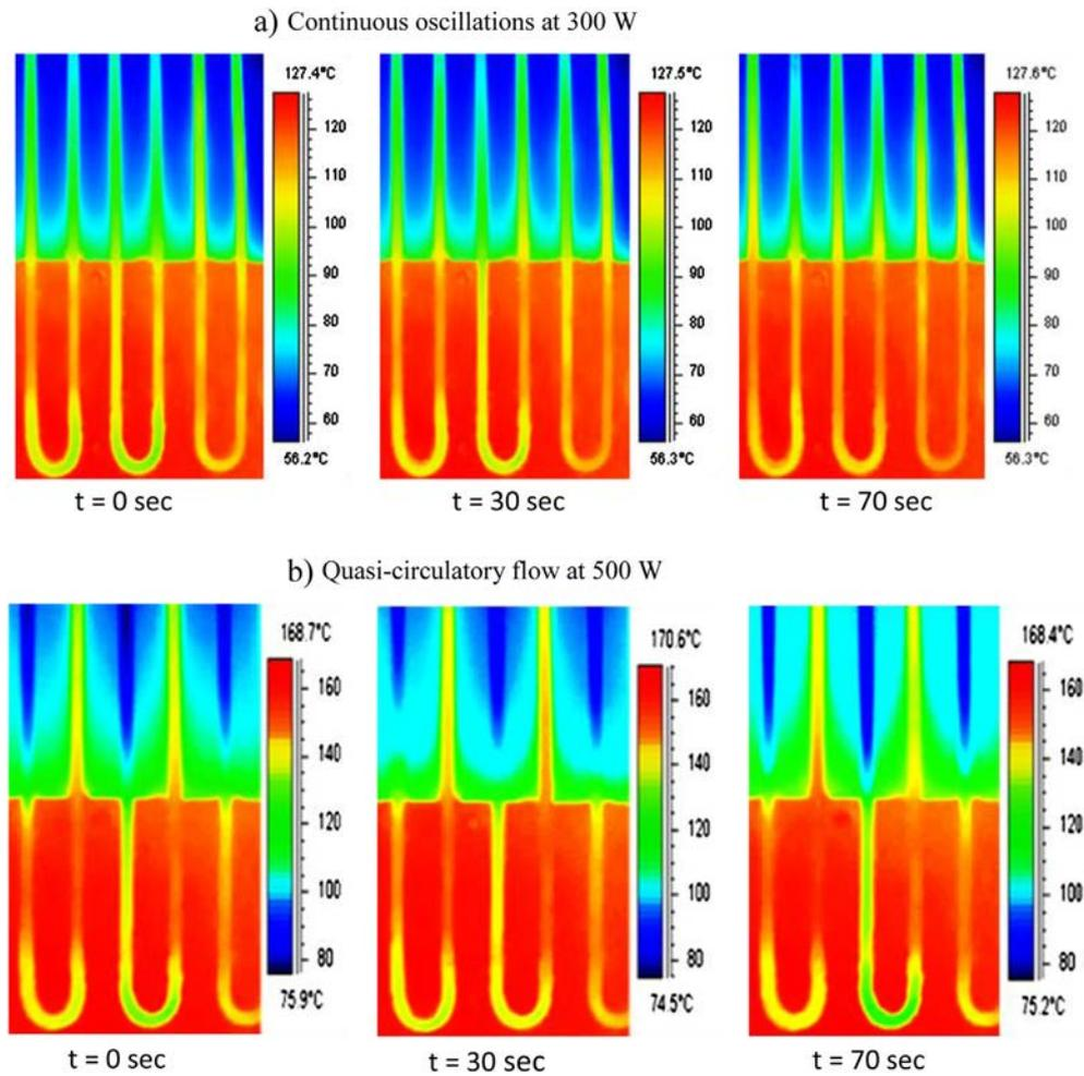
Fig. 10. Infra-red pictures of the evaporator at 300 W and 500 W operations, respectively.
