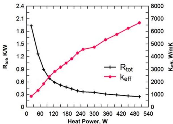
Fig. 11. Total thermal resistance and effective thermal conductivity of the PHP obtained at different input heat power.
