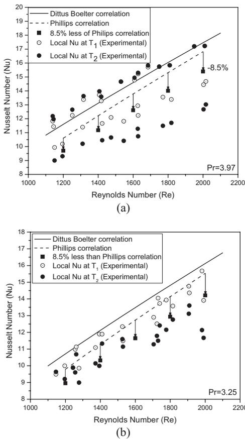
Figure 8. COMPARISON OF EXPERIMENTAL AND THEORETICAL Nu FOR TURBULENT FLOW (a) Pr 3.97 (b) Pr 3.25
