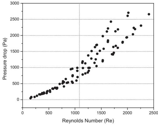
Figure 3. EXPERIMENTAL PRESSURE DROP vs FLOW Re
