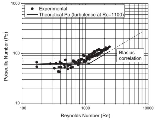
Figure 4.  $Po$  vs.  $Re$  FOR THE ARRAY
