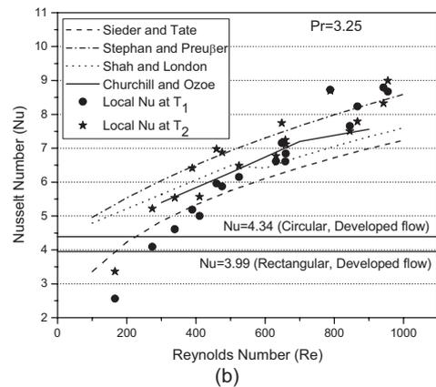
Figure 7. COMPARISON OF EXPERIMENTAL AND THEORETICAL VALUES OF Nu FOR LAMINAR FLOW (a) Pr = 3.97, (b) Pr = 3.25
