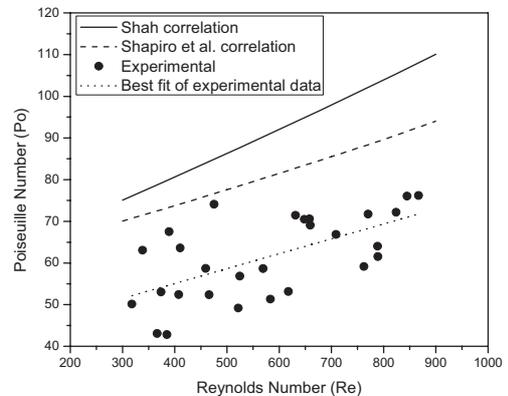
Figure 5.  $Po$  vs.  $Re$  FOR DEVELOPING LAMINAR FLOW
