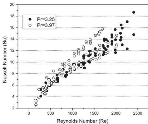
Figure 6.  $Nu_x$  vs. Re AT DIFFERENT LOCATIONS
