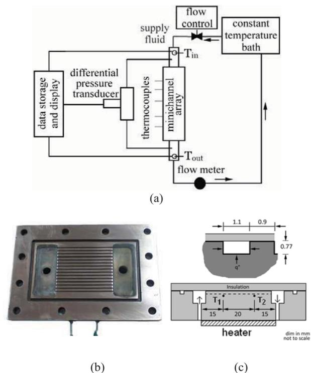
Figure 1. (a) SCHEMATIC LAYOUT OF THE EXPERIMENTAL SETUP (b) COPPER PLATE MINI-CHANNEL ARRAY (c) DETAILS OF THE MINI-CHANNEL ARRAY
