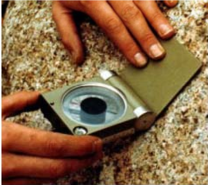
A geological compass to measure dip and direction of joint plane
