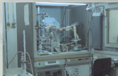
Diffractometer, Siemens D-500 (S2), with temperature chamber, TTK, and device for humidity controlled measurements
