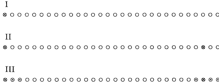
Figure 2. Snapshots of the failure process in a median strength ( N = 50 ) 1D HLLS \delta -bundle with 30 Weibull fibers for \rho = 10 and periodic boundary conditions. \bigcirc intact fibers, \otimes broken fibers and \odot first failures after instability.
