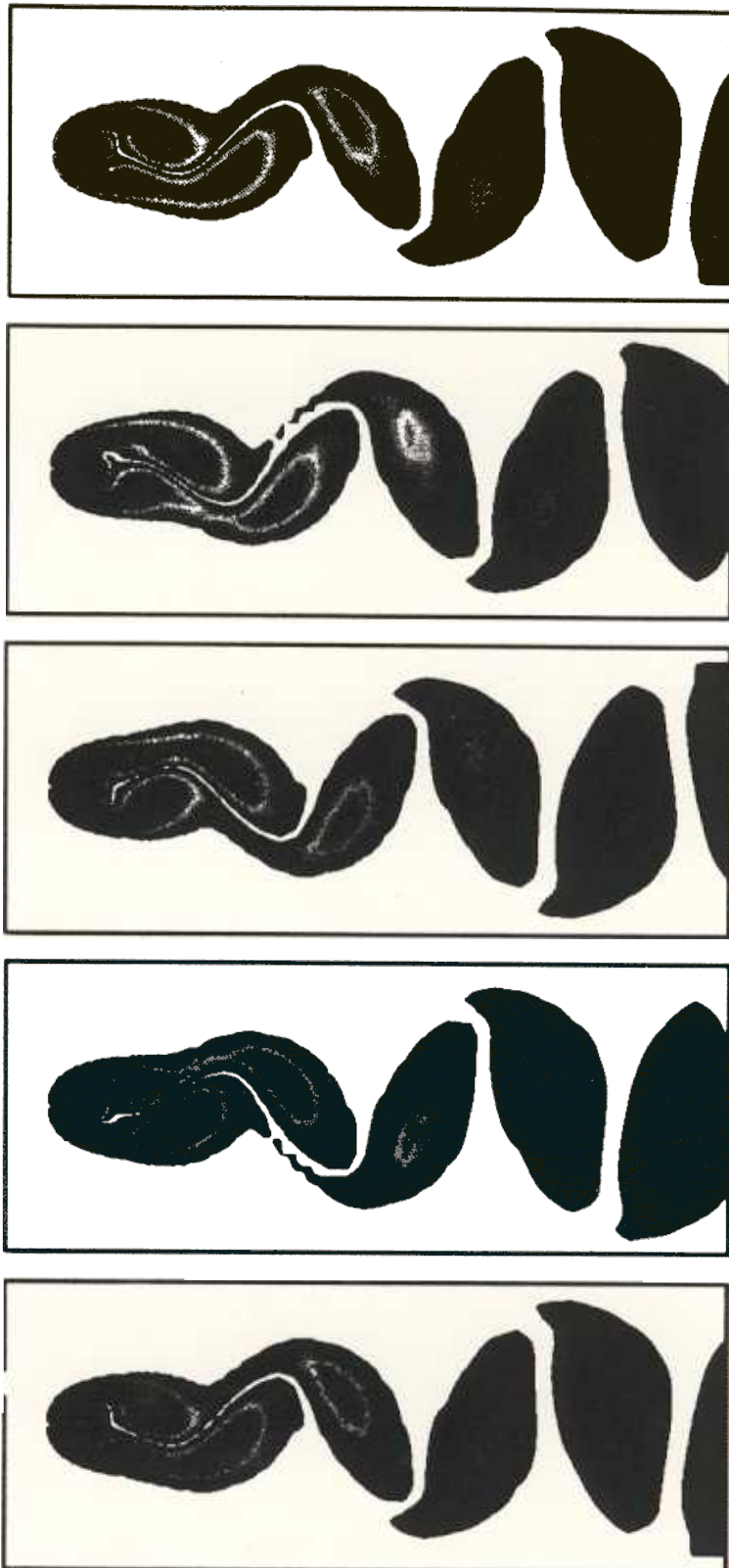
Plate I (Mittal et al. ). Flow past a fixed cylinder at Re = 100 : vorticity at various instants during one period of the lift coefficient
