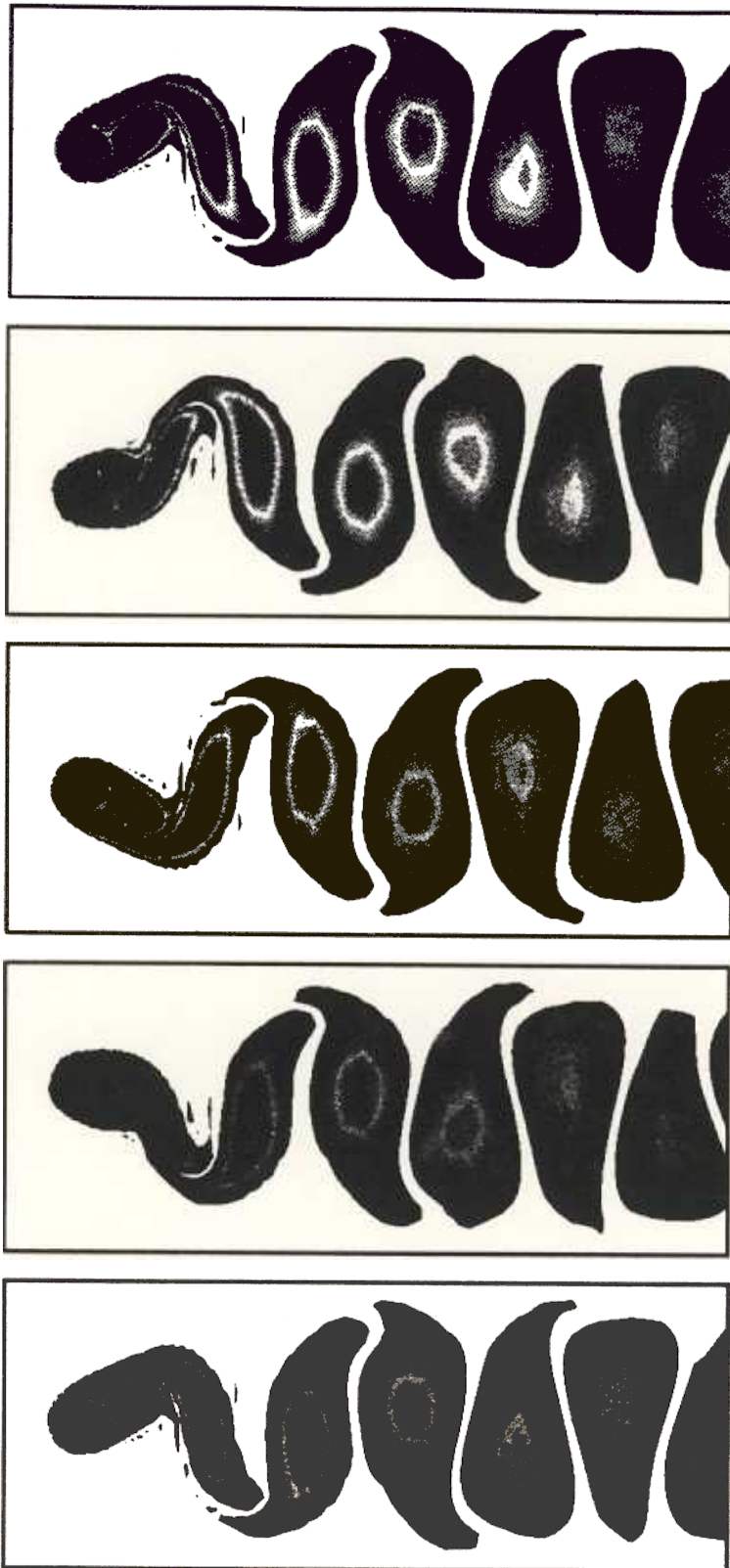
Plate V (Mittal et al. ). Flow past a vertically oscillating cylinder at Re = 324 : vorticity at various instants during one period of the cylinder motion
