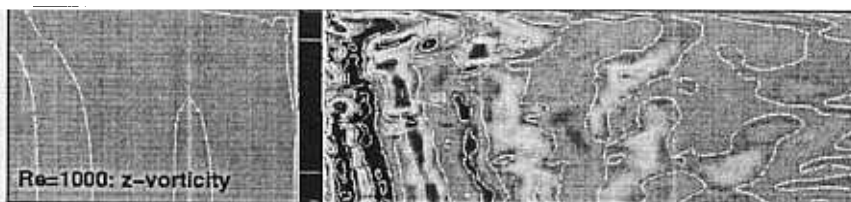
Figure 4: 3D flow past a circular cylinder of aspect ratio 16. Top wall is no-slip and
