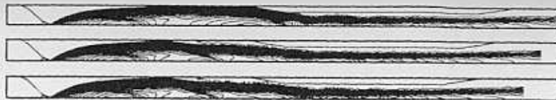
Figure 12. Supersonic flow through a wind-tunnel, A_2/A_1 = 0.7 , p_o/p_o = 22 , L_s = 2 : the iso-mach contours for various values of the length of the constant area section of the diffuser (from top to bottom) L_c = 8.8, 8.0 and 7.2
