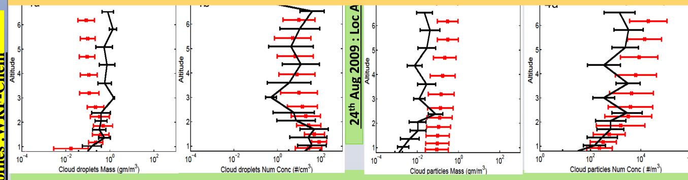
Comparison of vertical profiles from CAIPEEX (Black line) flight measurements with WRF Chem (Red dots) simulated (a)mean cloud droplet mass conc., (b)mean cloud droplet number conc., (c)mean cloud particle mass conc. and (d)mean cloud particle number conc. on 24<sup>th</sup> Aug (Figure 4) and 25<sup>th</sup> Aug (Figure 5). Altitude is in Km.
