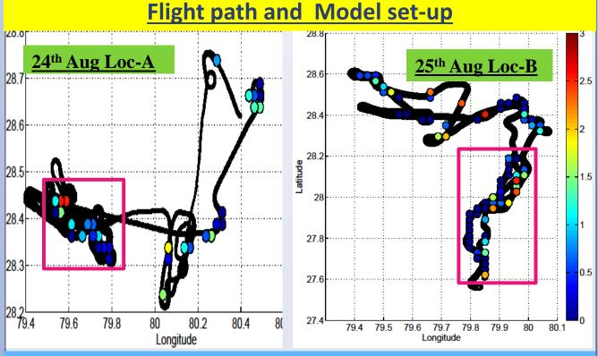
Figure 1 shows the flight path on 24<sup>th</sup> and 25<sup>th</sup> in black dots. The colored dots are total hydrometeor mass conc. (g/cubicmetre). Two regions (pink boxes ) are studied where aircraft measurements are present upto 7 km altitude.
