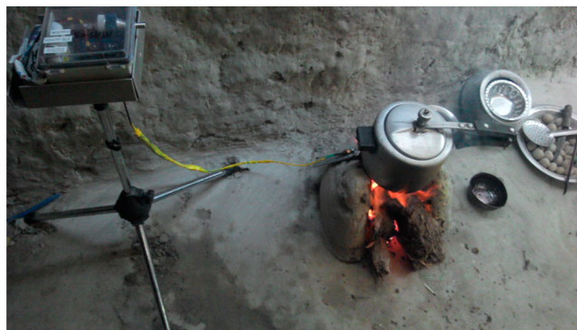
Figure 1. Image taken from BC_PS. Sampler located in the breathing zone. Stove instrumented with WiCS cookstove sensor (yellow cable) to track the cooking time and fuel usage.
