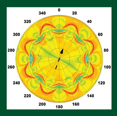
Penetration and screening of perpendicularly launched electromagnetic waves through bounded supercritical plasma confined in multicusp magnetic field by I. Dey and S. Bhattacharjee
