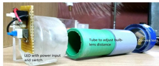
Figure 4.4. Fabricated collimated light source.
