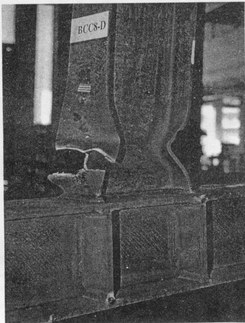
Fig. 16 Fracture of the beam flange in the buckled zone (BCC8)
