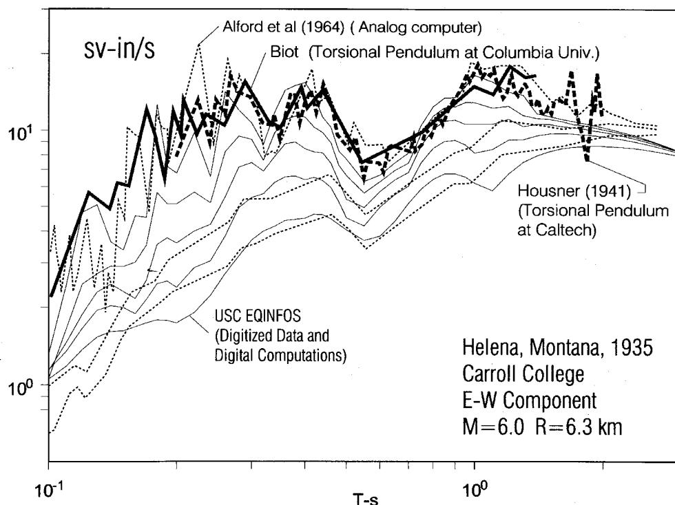
Fig. 4 Comparison of relative velocity response spectrum amplitudes for E-W component of strong motion recorded at Carroll College, during Helena, Montana earthquake of 1935 (spectra computed by torsional penduli of Biot and Housner (damping not specified) are compared with spectra computed by analog computer (damping values 0, 0.10, and 0.20), and digital computer (for five damping values 0, 0.02, 0.05, 0.10, and 0.20; Lee and Trifunac, 1987))
