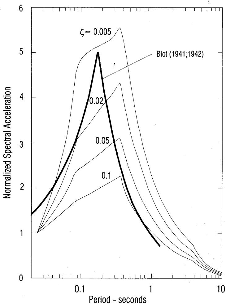
Fig. 8 Comparison of Biot (1941, 1942) “standard spectrum” (heavy line) with regulatory guide 1.60 spectrum (USAEC, 1973)
