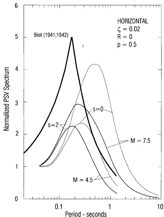
Fig. 10 Comparison of Biot (1941, 1942) “standard spectrum” (heavy line) with spectral shapes, which depend upon magnitude ( $M = 4.5$  and  $7.5$ ) and geological site conditions ( $s = 2$  for basement rock and  $s = 0$  for sediments), for average spectral amplitudes ( $p = 0.5$ ), at zero epicentral distance ( $R = 0$ ) and for 2 percent of critical damping ( $\zeta = 0.02$ ; Trifunac, 1978)
