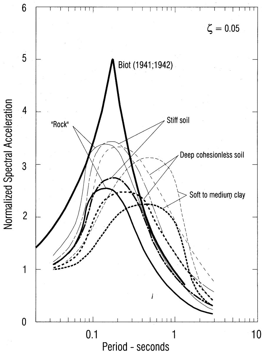
Fig. 9 Comparison of Biot (1941, 1942) "standard spectrum" (heavy line) with average (heavy lines) and average plus standard deviation spectra (light lines) of Seed et al. (1976) for four soil site conditions
