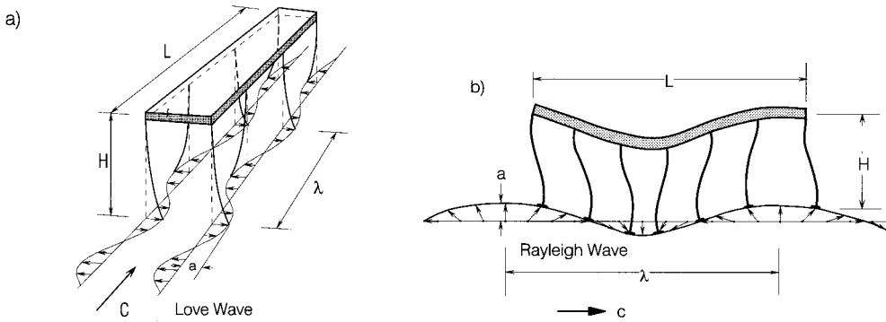
Fig. 11 (a) Deformation of columns in a two-degree-of-freedom system, during out-of-plane response, excited by Love waves, (b) Deformation of columns in a long structure during in-plane response and excited by Rayleigh waves
