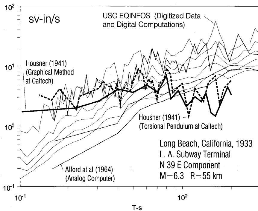
Fig. 5 Comparison of relative velocity response spectrum amplitudes for N39E component of strong motion recorded at Los Angeles Subway Terminal, during Long Beach, California earthquake of 1933 (spectra computed by graphical method (zero damping), torsional pendulum (damping not specified), analog computer (damping values 0, 0.10, and 0.20), and digital computer (for five damping values 0, 0.02, 0.05, 0.10, and 0.20; Lee and Trifunac, 1987))
