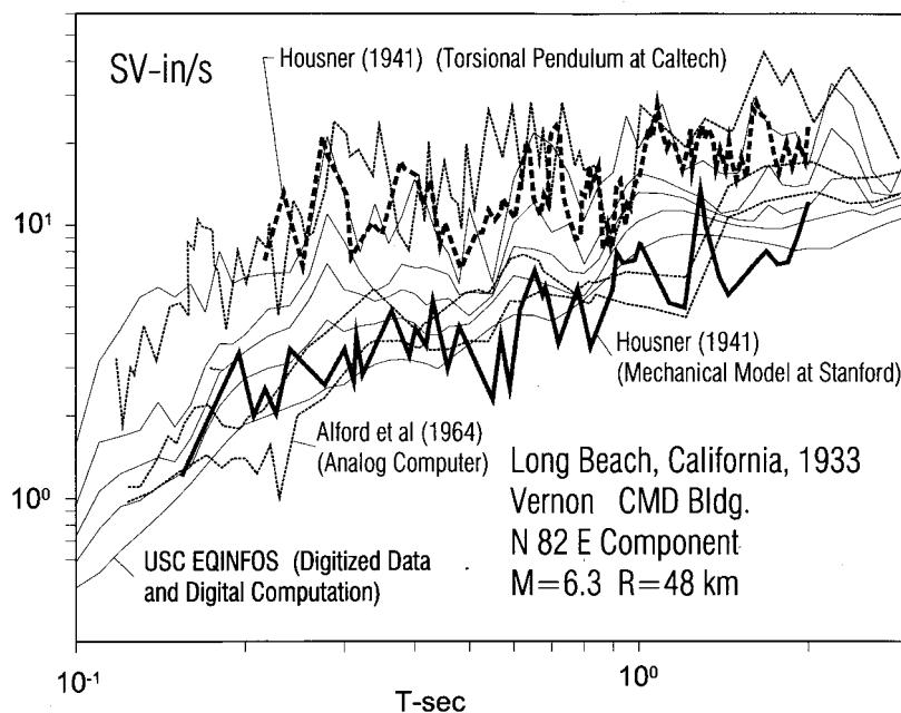
Fig. 6 Comparison of relative-velocity response spectrum amplitudes for N82E component of strong motion recorded at Vernon, CMD Building, during Long Beach, California earthquake of 1933 (spectra computed by mechanical model at Stanford (damping not specified), torsional pendulum at Caltech (damping not specified), analog computer (three damping values 0, 0.10, and 0.20), and digital computer (for five damping values 0, 0.02, 0.05, 0.10, and 0.20; Lee and Trifunac, 1987)).
