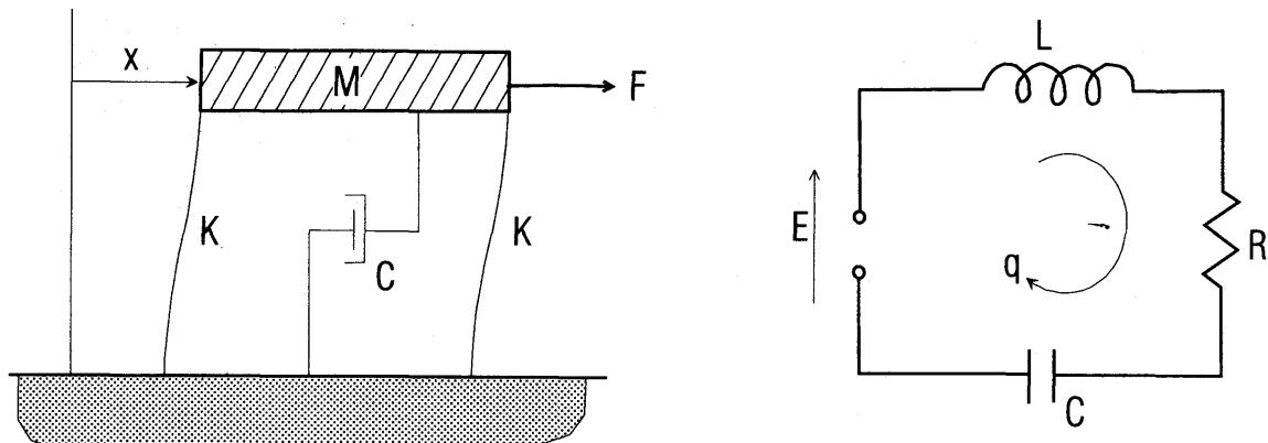
Fig. 2 Basic electro-mechanical analog (redrawn from Alford et al. (1964))
