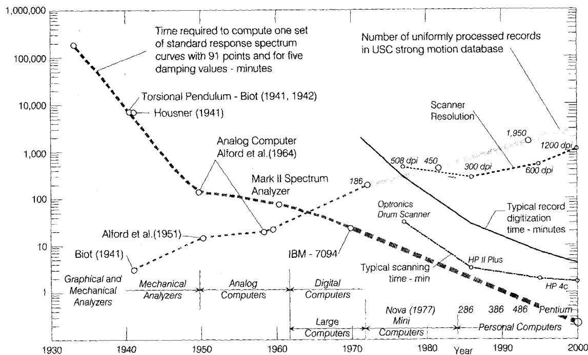
Fig. 1. Trends in the capabilities of accelerogram digitization and data processing, between 1970 and 2000: time required to compute one set of standard response spectrum curves (in minutes), and the cumulative number of accelerograms in strong-motion data bases (light dashed line for the period prior to 1970), and in the uniformly processed strong-motion data bases (wide gray line for the period after 1970)
