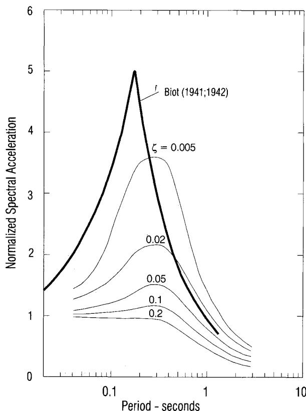
Fig. 7 Comparison of Biot (1941, 1942) "standard spectrum" (heavy line) with average spectrum of Housner (1959, 1970)
