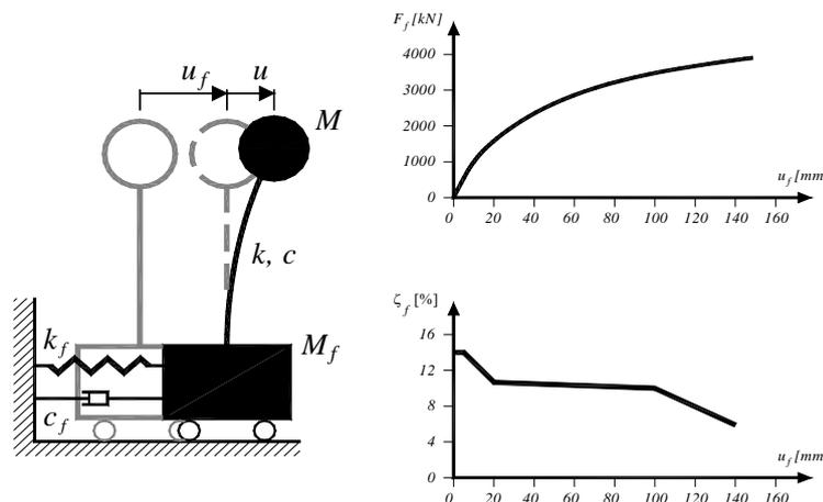
Fig. 21 2-DOF equivalent model for the retrofitted system
