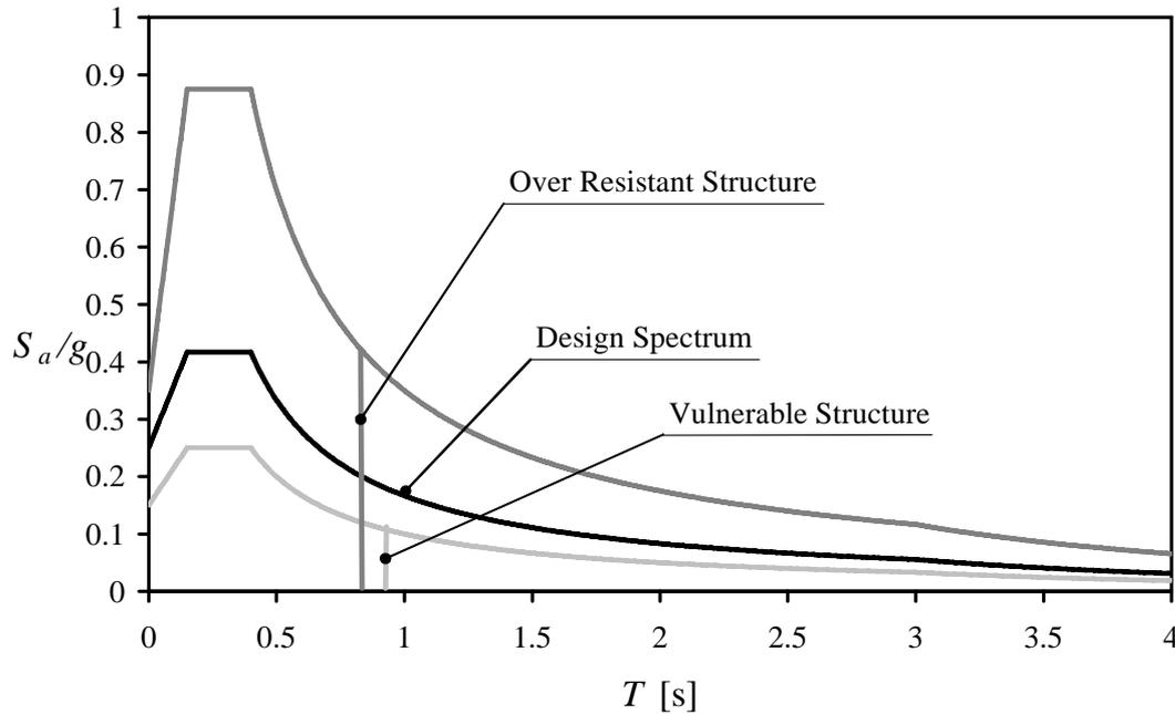
Fig. 3 Comparison between seismic resistance and seismic demand
