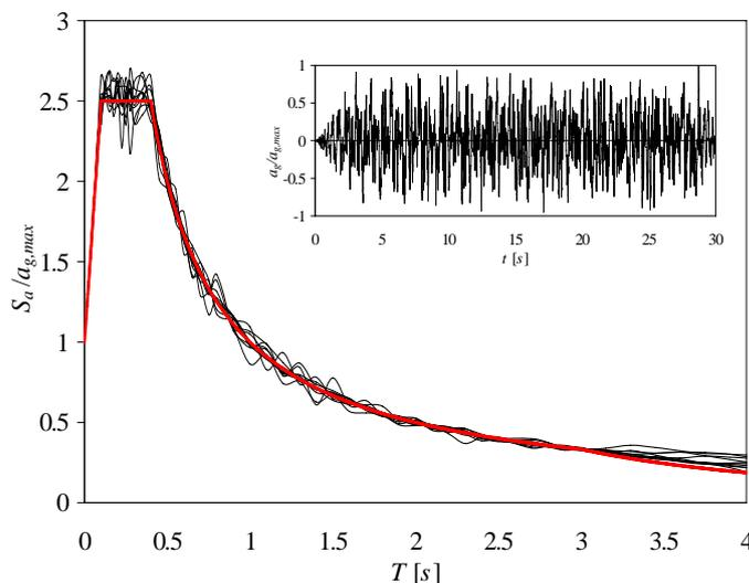
Fig. 24 Response spectra of 12 spectrum-compatible acceleration samples
