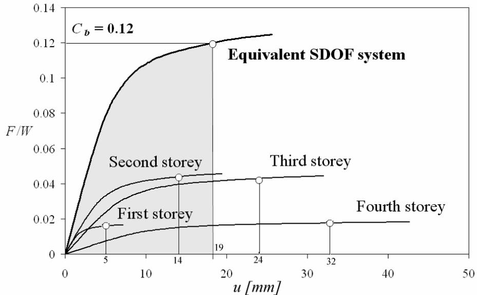
Fig. 12 Evaluation of the equivalent SDOF system on the basis of the storey force-displacement (push-over) curves
