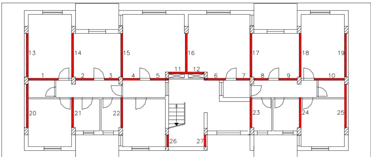
Fig. 19 Deformability reduction by reinforced concrete thin walls; first storey
