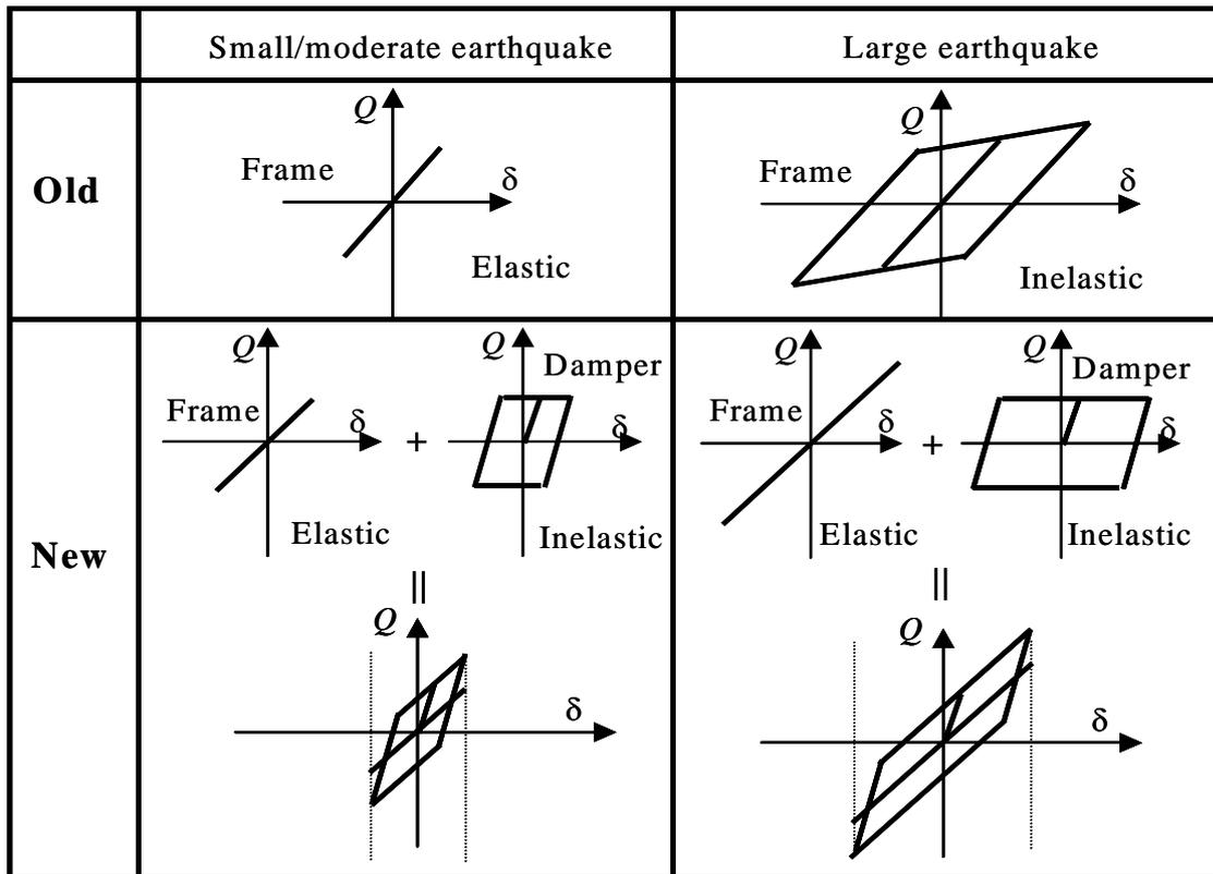
Fig. 9 Comparison of old system with new system (Huang et al., 2001) on a constitutive level
